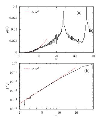
Figure 6. Density of states measured on the (1,1,1) cut, data from the molecular dynamics simulation [1]. (a) Note the prominent van Hove singularities corresponding to the longitudinal and transverse projected modes. Panel (b) plots the integrated density of states on a log-log scale, compared with the theoretical form  $\omega^4$ .
