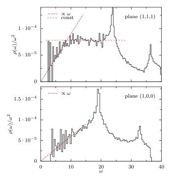
**Figure 7.** Density of states divided by  $\omega^2$ , projected on two different planes. The resulting curves depend on the projection plane: In the case (1,1,1) the expected regime in  $\rho \sim \omega^3$  is seen for  $\omega < 10$ ; a plateau is observed for  $10 < \omega < 20$ . The form  $\rho \sim \omega^3$  fits over a larger range of  $\omega$  for the case (1,0,0).
