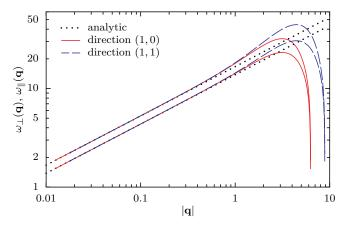
**Figure 1.** Longitudinal and transverse fluctuations of an isotropic system projected to the two-dimensional plane (1,0,0). The result is compared to the long-wavelength limit (dotted line) predicted in Eq. (5).  $L=512, \lambda=70, \mu=95, \gamma=0$ .
